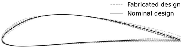
Fig. 3 An example of nominal airfoil design and its corresponding fabricated designs
